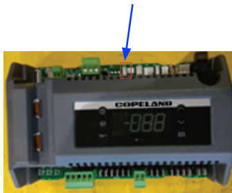
Jumper to be installed
